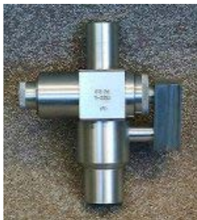
Figure 4-1: Very Sharp Cut Cyclone (VSCC) Used for PM2.5 Sampling
