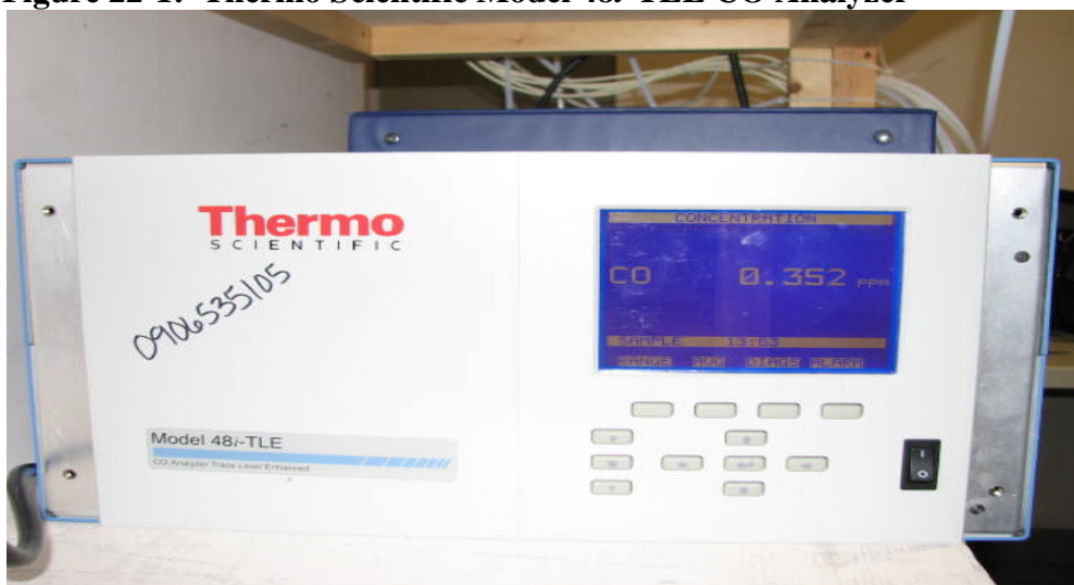
Figure 22-1: Thermo Scientific Model 48i-TLE CO Analyzer
