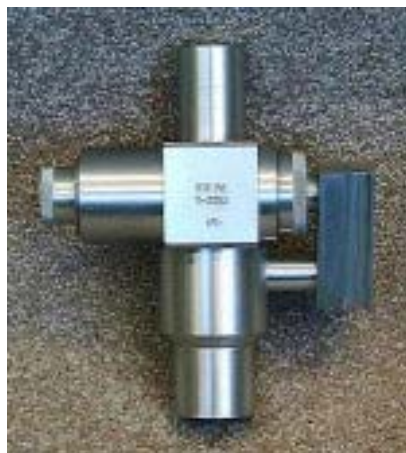
Figure 5-1: Very Sharp Cut Cyclone (VSCC) Used for PM2.5 Sampling
